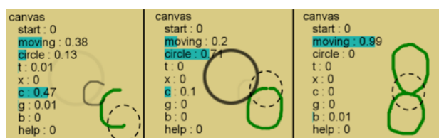
Figure 10.13: Screenshots of the canvas interactor as user draws a figure 8. The “c” and circle gesture share a common prefix. Dotted line indicates finger location. Left: Initially a ‘c’ gesture is most likely (probability 0.47). Feedback indicates that c is the most likely interpretation, though a circle is possible. Middle: The system becomes confident that the gesture is a circle, reflecting this in feedback (also evident in state distribution). Right: As the user completes the figure 8, the canvas believes the user is painting and removes all gesture feedback.
